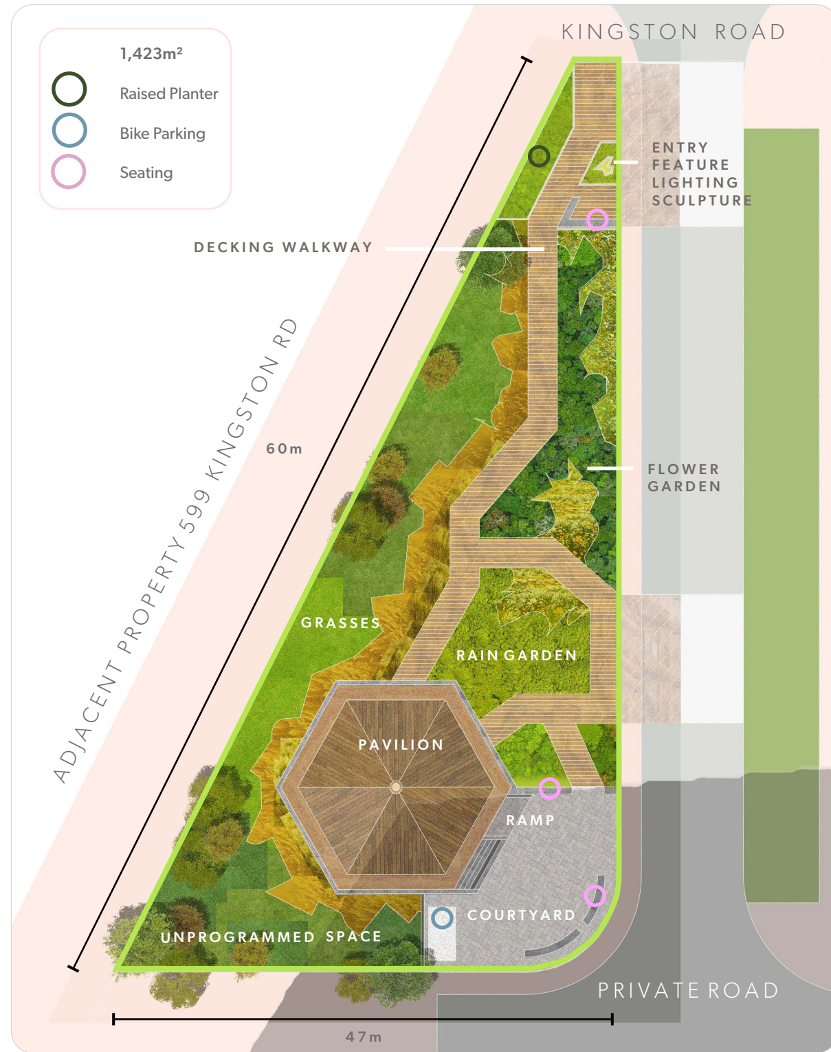
Figure 8: Park 1 Plan - Please note that all figures are approximate and subject to change.
