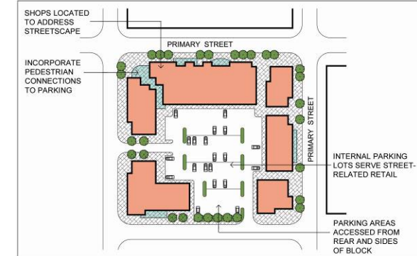
Parking court at interior of a commercial block
