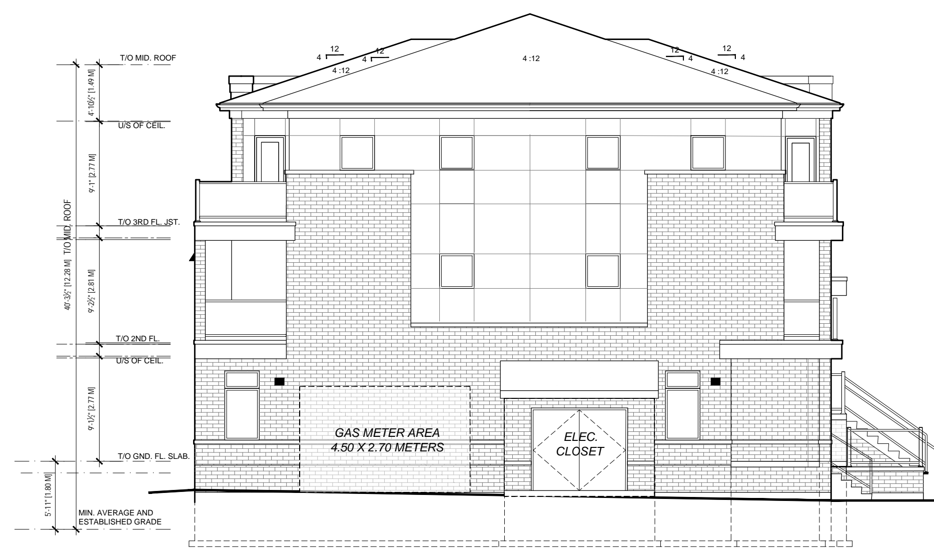
BLOCK 9 WEST ELEVATION 1:100 5-PLEX STACKED TOWNS
