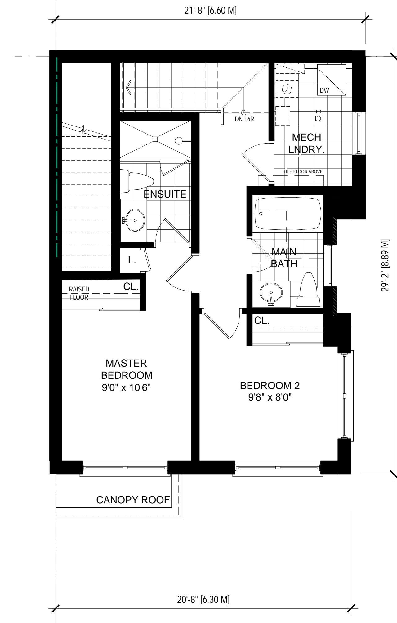
MODEL SF-E3 SECOND FLOOR PLAN SCALE: 1:50
