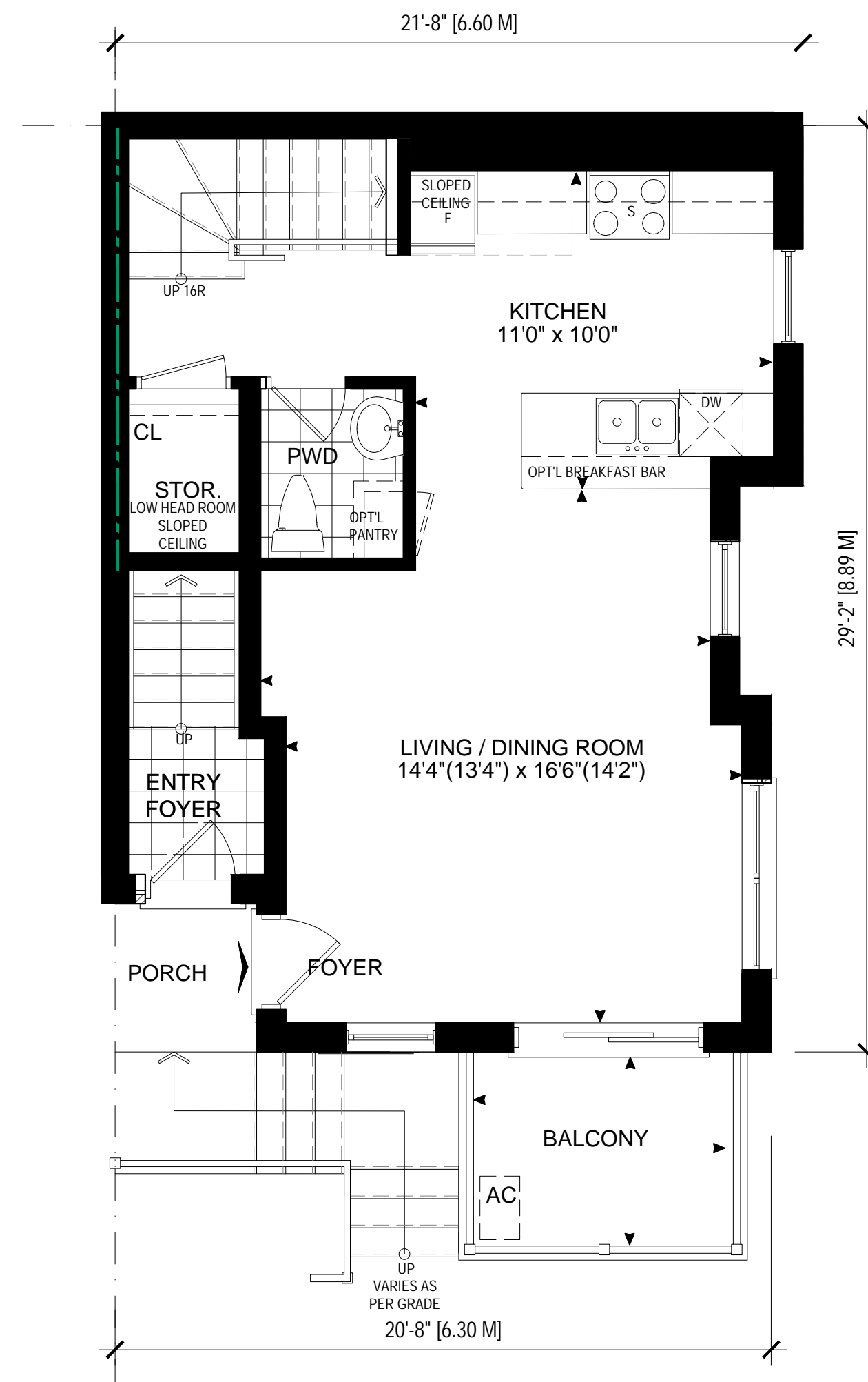
MODEL SF-E3 GROUND FLOOR PLAN SCALE: 1:50
