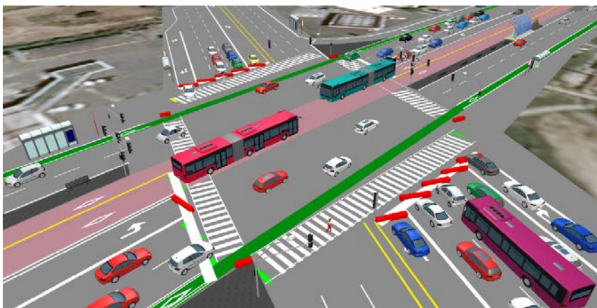
FIGURE 31: DURHAM-SCARBOROUGH BRT AT KINGSTON ROAD AND WHITES ROAD
