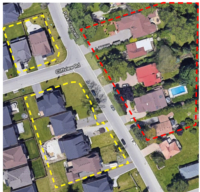
Figure 16: Google map aerial of Cliffview Road and Park Crescent showing the replacement housing (yellow) differs in side yard setback and separation distance between houses as compared to original dwellings (red).
