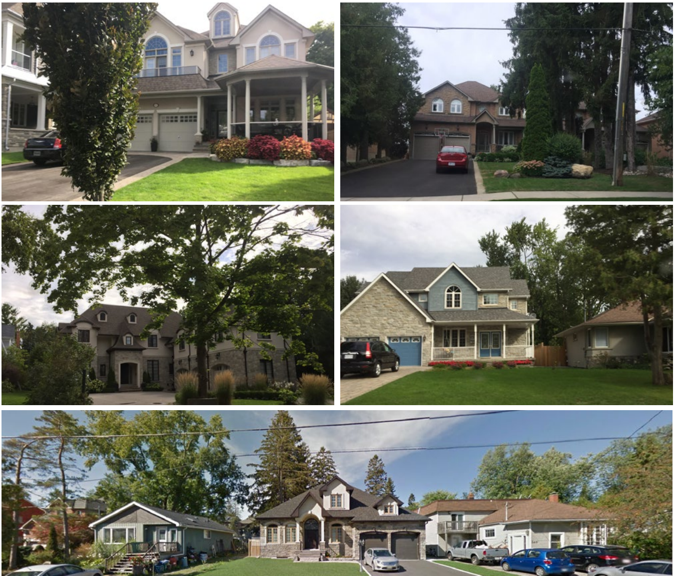
Figure 3: Images of infill and replacement housing within Pickering's Focus Neighbourhoods that respects existing character through design elements ranging from height, garage placement, setback, landscaping, roof slope, and tree protection.
