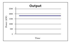
OptiSlip® allows the rotor speed to vary within a range of approximately 10 percent in relation to nominal rpm. This minimizes both unwanted fluctuations in the output to the grid supply and the loads on the vital parts of the construction.
