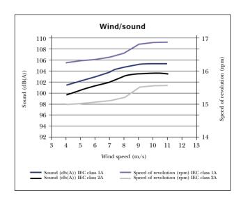
The sound output level can be adjusted by varying the revolution speed of the turbine as illustrated in the figure above. In practice, this means that, for example, the sound level recorded at a distance of 340 m (hub height 78 m) can be reduced from 44.5 to 40.4 dB(A) – i.e. by more than half the recorded level.
