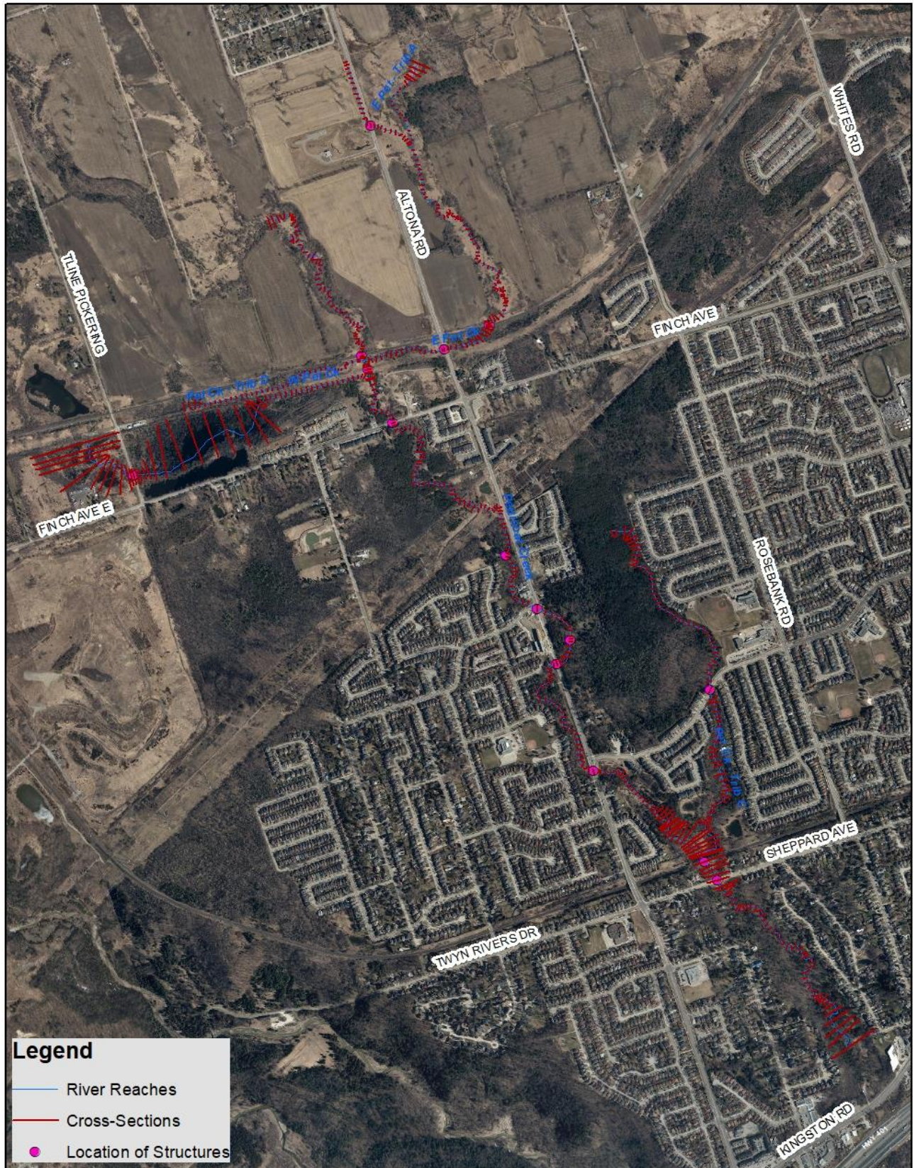
Figure 11 Location of 1D cross-sections and structures
