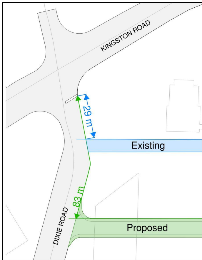
Figure 8-4: Dixie Road Access – Intersection Distances
