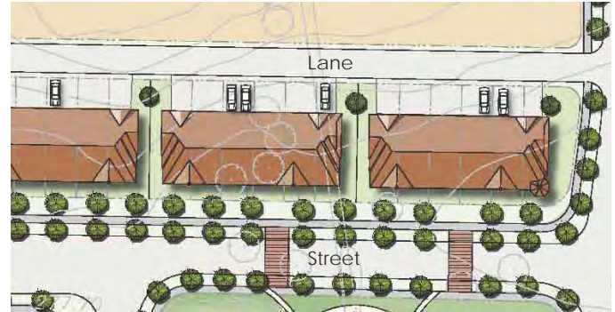
Lane-access garages minimizes the number of driveways across the sidewalks, and remove the dominance of the car from the streetscape.
