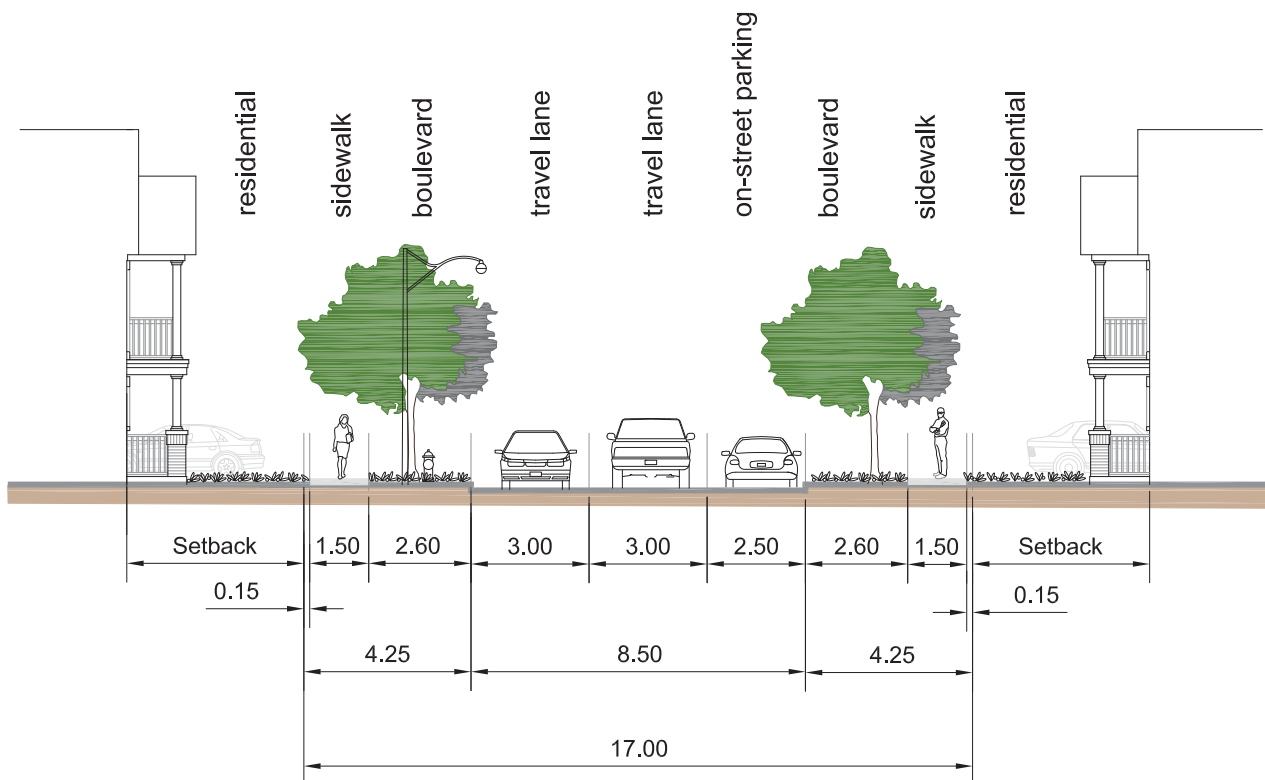
Typical Cross Section for Local Road - Double-loaded road with on-street parking without rear lanes 17.0 metre Right-of-way
