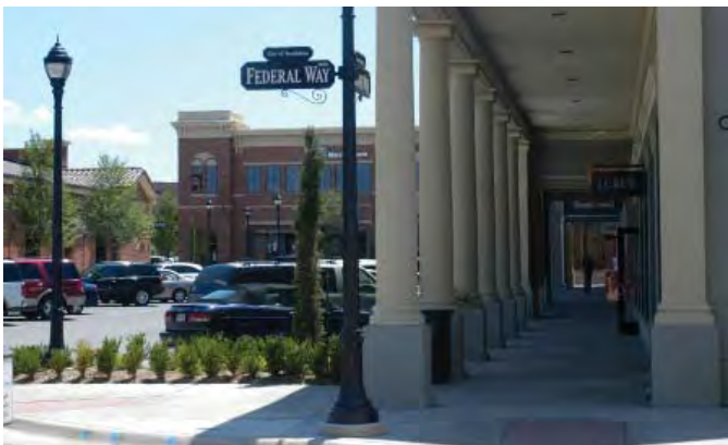
Weather protection is integrated into the design of the building for pedestrian comfort, and provides access to parking areas.
