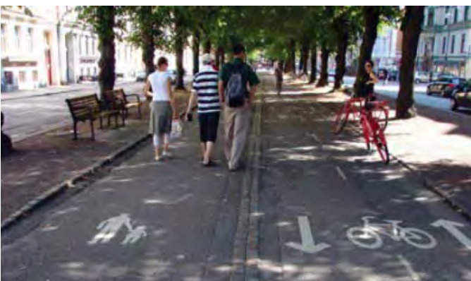
Clear demarcation of pedestrian and cycling lanes through road painting and markings.
