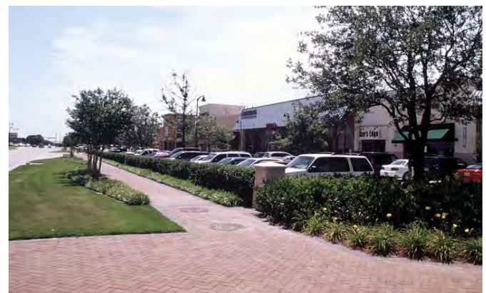
Lowered parking surfaces and landscaped buffers help screen parking areas from street view.
