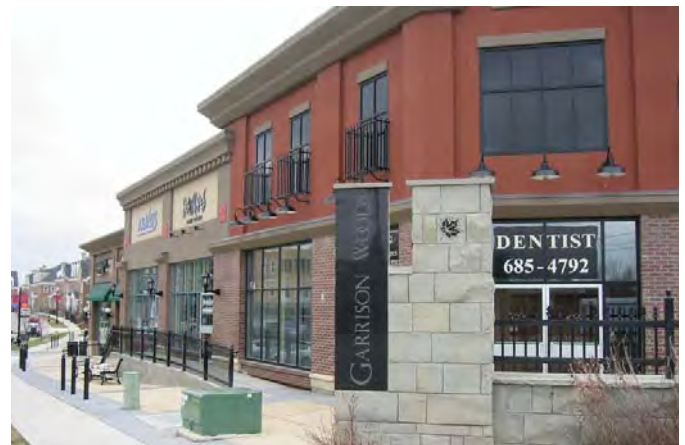
The main entry door and windows should be located along the Pedestrian Predominant Street to create a consistent block face of a minimum 75%.
