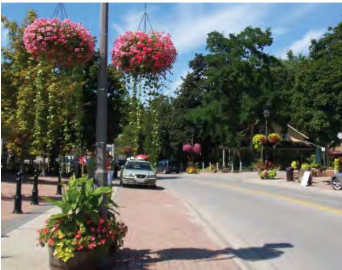
Rolled curbs and special paving should be provided in high pedestrian areas, such as Pedestrian Predominant Streets.
