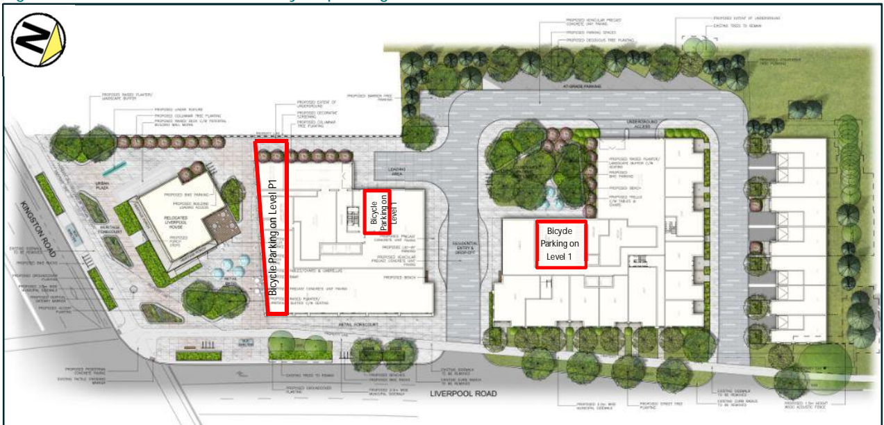
Figure 10.3: On-site and off-site bicycle parking locations
