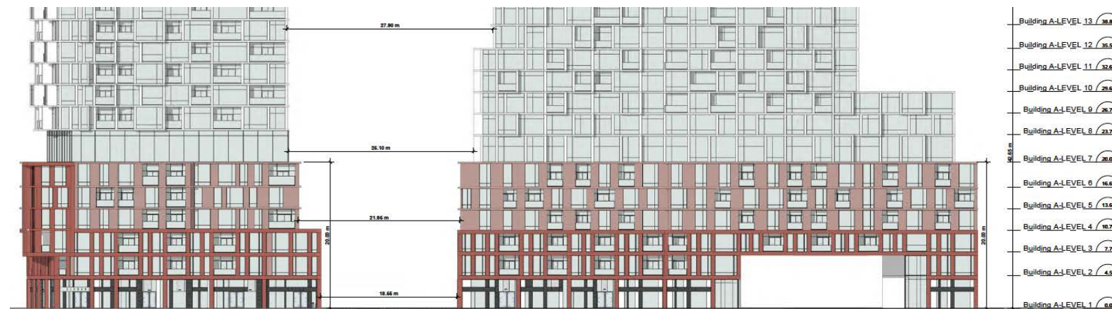
> Elevation showing building separation and setbacks
